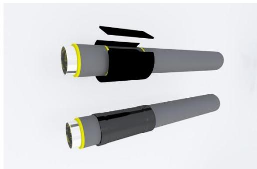
**NOVORAD-ST heat-shrinkable wraparound sleeve** refers to a heat shrinkable band coated with a hot-melt adhesive. The sleeve is used along with NOVORAD-ZK adhesive closure patch and NOVEP epoxy primer. The full set provides a single anticorrosive protection system covering main body of a pipe.
