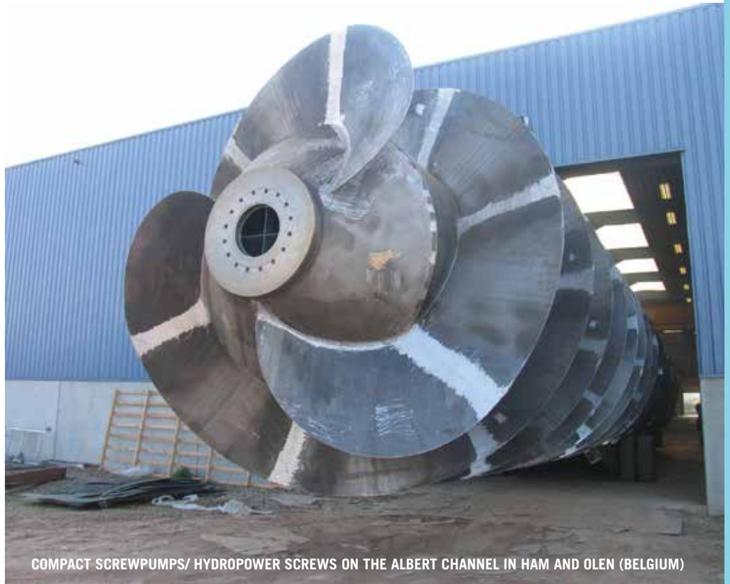
COMPACT SCREWPUMPS/ HYDROPOWER SCREWS ON THE ALBERT CHANNEL IN HAM AND OLEN (BELGIUM)
