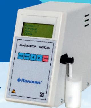
**Measured parameters (8):** Fat, Protein, SNF (Solids-non-Fat), Total Solids, Lactose, Density, Added Water, Freezing Point, Temperature
