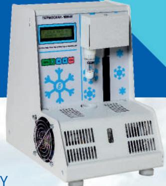
**APPLICATION:** measuring of freezing point of milk
