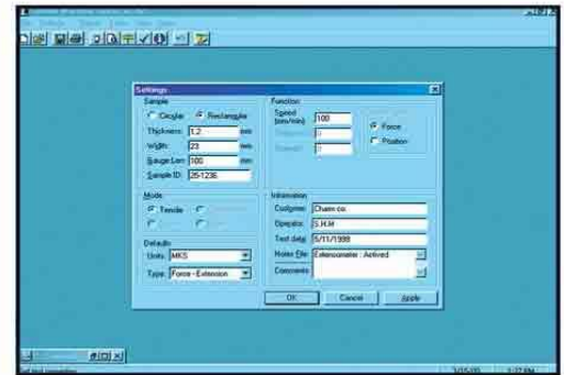
Entering Shape & Dimensions of Sample and Test Parameters
