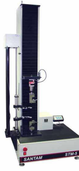
STM-5 with Roller Grips & Extensometer
